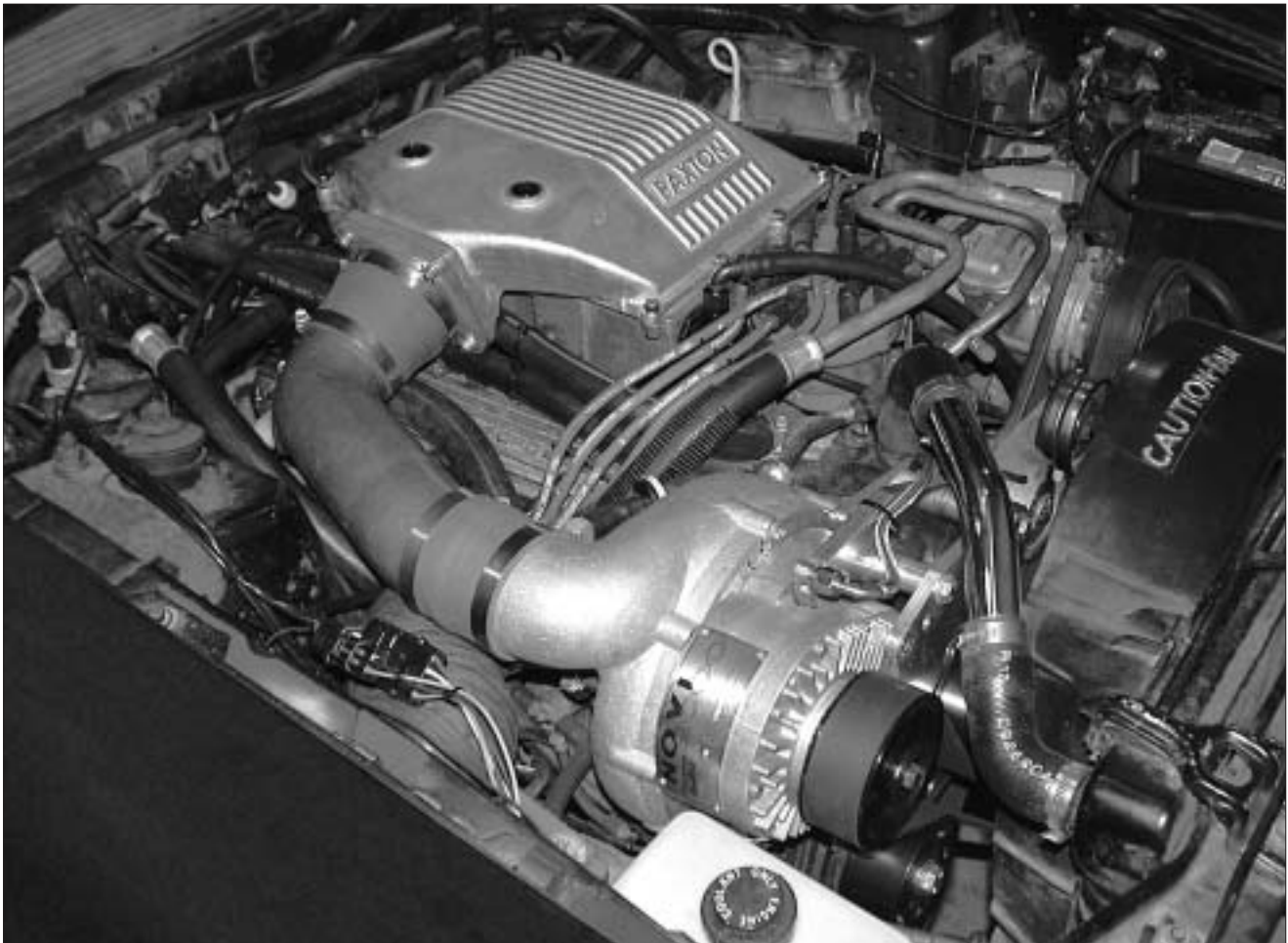
Completed Installation on a Carbureted 5.0L Ford Mustang Motor
